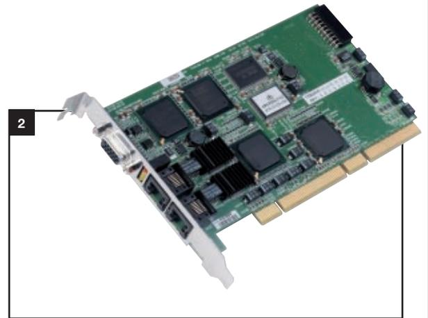
**2.** Two Port AFDX/ARINC664 test, simulator and monitor module for PCI
